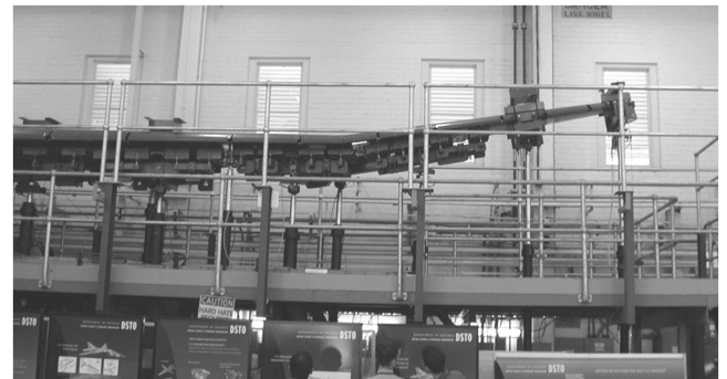
Fig. 11 F-111 wing in full-scale fatigue testing [26].
